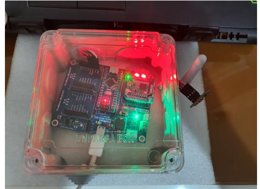
Figure 1. Physical prototype of the wearable sensor unit, including MAX30102 sensor, Arduino Nano, LED indicator, and buzzer.
