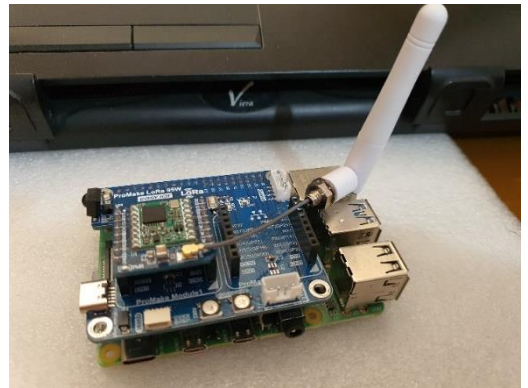
Figure 2. Raspberry Pi 4B and connected LoRa module used as the central edge node
